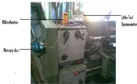
Figure2. Experimental setup for measuring average chip-tool interface Temperature using Tool-work thermocouple technique [16]
